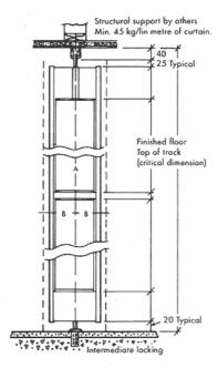
A. Panel width available 150mm or 300mm B. 175mm clearance from centre line of curtain to wall or column for 300 panel. 100mm minimum clearance from centre line of curtain to wall or column for 150 panel.
